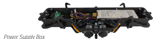
Power Supply Box
